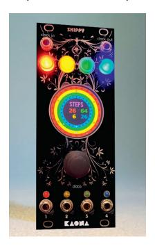
Skippy is a polyrhythmic (linear and logarithmic) matrix and non-matrix sequencer that offers four completely independent (but synchronized) tracks.
